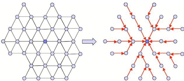
Figure 1: In response to a message originating from  $v_{root}$  (dark blue; left), child vertices respond to their respective parent vertices; the accumulated message paths of all responses form a spanning tree subgraph (right).
