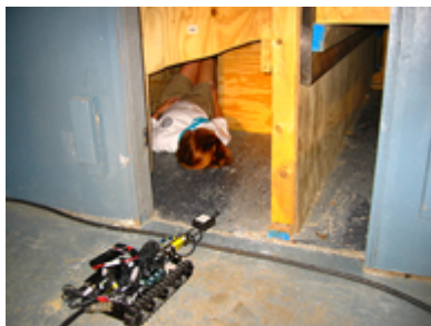
Robot with vital sign sensors being tested at the University of South Florida
