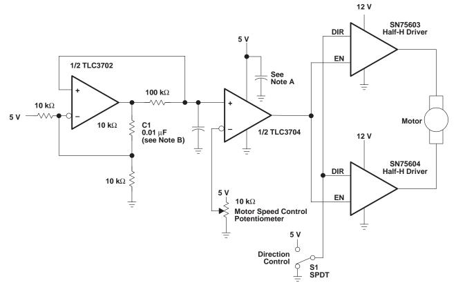
NOTES: A. The recommended minimum capacitance is 10  $\mu$ F to eliminate common ground switching noise.
