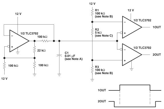
NOTES: A. Adjust C1 for a change in oscillator frequency where:  $1/f = 1.85(100 \text{ k}\Omega)\text{C1}$
